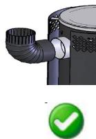
5. Non crimped end of exhaust elbow is designed to slide over the heater exhaust collar
